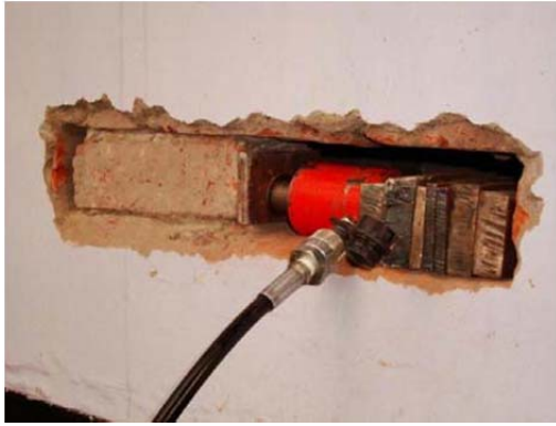
Fig A. I.3. Test Setup for In-Situ Shear Test
