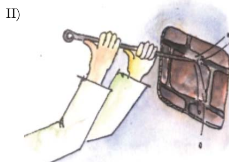
Figure 4.39 Removing stone by small rod
