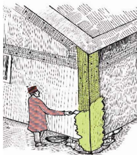
Figure 4.11 Plastering vertical WWM belt using cement plaster (Adapted from: UNDP, UNESCO & GOI, 2007)
