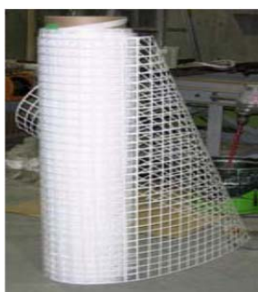
Figure 4.15 PP band mesh (Source: Meguro and Mayorca)
