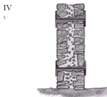
Figure 4.41 Placing steel bar and filling concrete
