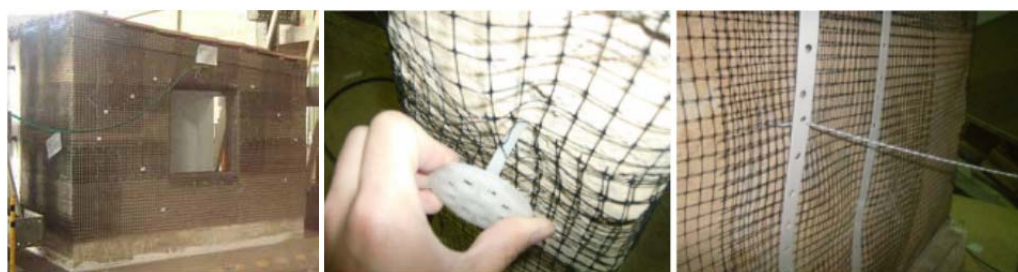
Figure 4.24 Reinforced house with geomesh
