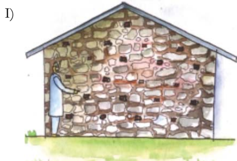
Figure 4.38 Marking points for bond elements
