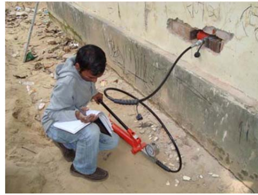
Fig A. I.3. Test Setup for In-Situ Shear Test
