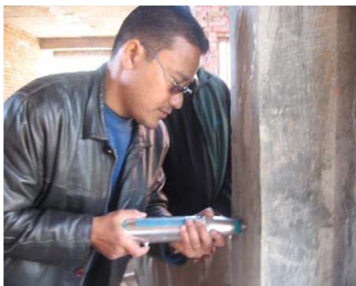
Fig A.I. 1.(a)Use of Rebound Hammer
